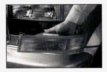
Completely remove the sidemarker/turn signal lamp by pulling out the assembly and disconnecting the side marker/turn signal lamp sockets from the lamp.
